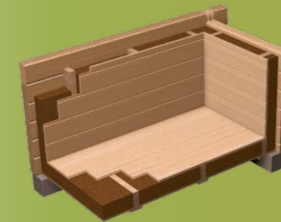
Thermo wall inside
