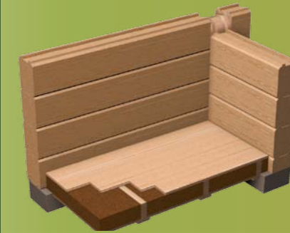
Massive log wall
